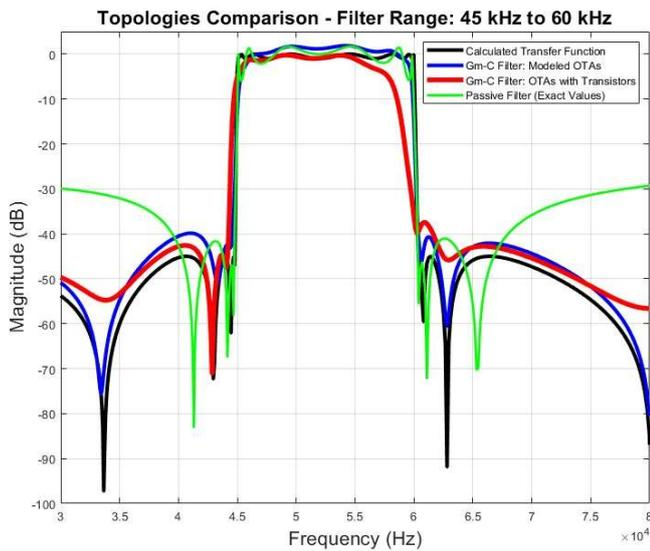
Fig. 6. Comparison of different responses for the 45-60 kHz filters.
