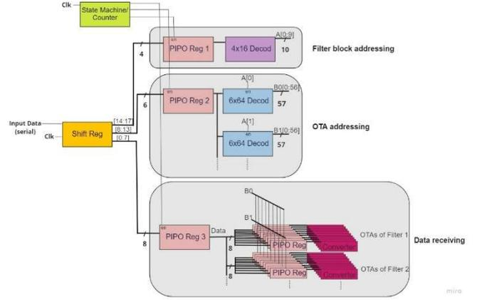
Fig. 5. Biasing/tuning block diagram.
