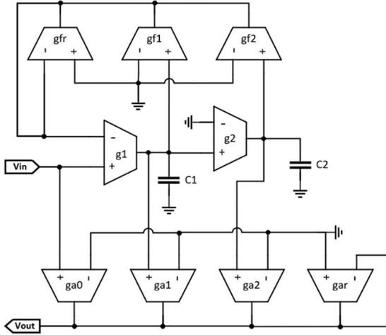
Fig. 2. A second-order FLF Gm-C filter section.
