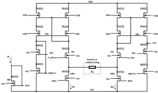
Fig. 3. The proposed OTA, with the source-degeneration scheme.
