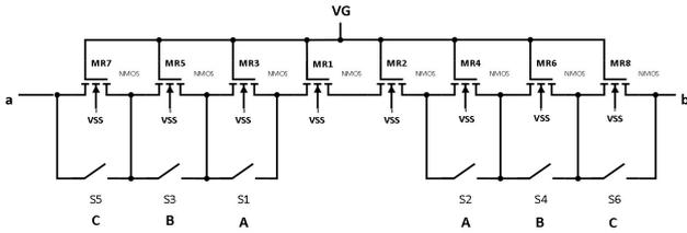
Fig. 4. Detail on the resistive string, implemented by MOSFETs in triode region.
